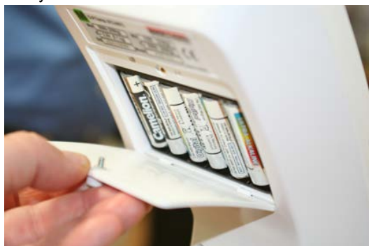
Figure 2-4. Batteries in Battery Chamber
